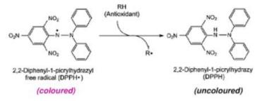
**Figure 9.** Reaction between an antioxidant and the DPPH free radical (Moon and Shibamoto, 2009).
