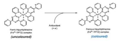
Figure 10. Reduction of Fe3+ into Fe2+ by an antioxidant (Moon and Shibamoto, 2009).
