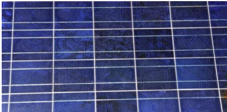
Figure II.9 : Traces d'escargot ‘Snail tracks’
