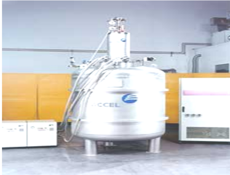
Figure 1-6. Superconductivity bobbin for energy storage of 2MJ (With autorisation of « ACCEL Instruments ») [7].
