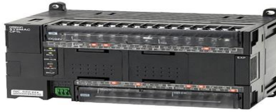
Figure I. 2: Automate programmable industriel mono bloc.
