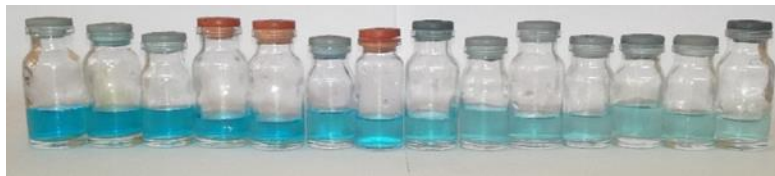
Figure 5: Decoloration test of the BM solution conducted in the presence of the F1 film [19].
