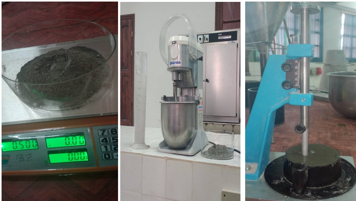
Figure III.22 : Essai de consistance de ciment.
