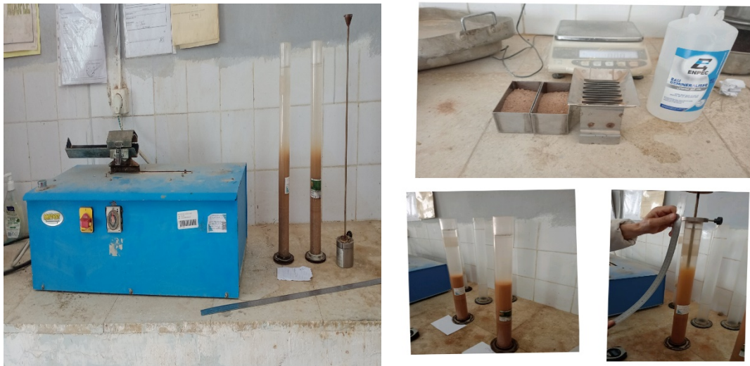
Figure III.13 : Equivalent de sable.
