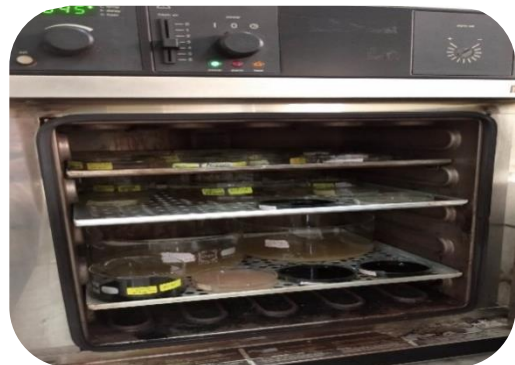
(f) Evaporation des solvants.
