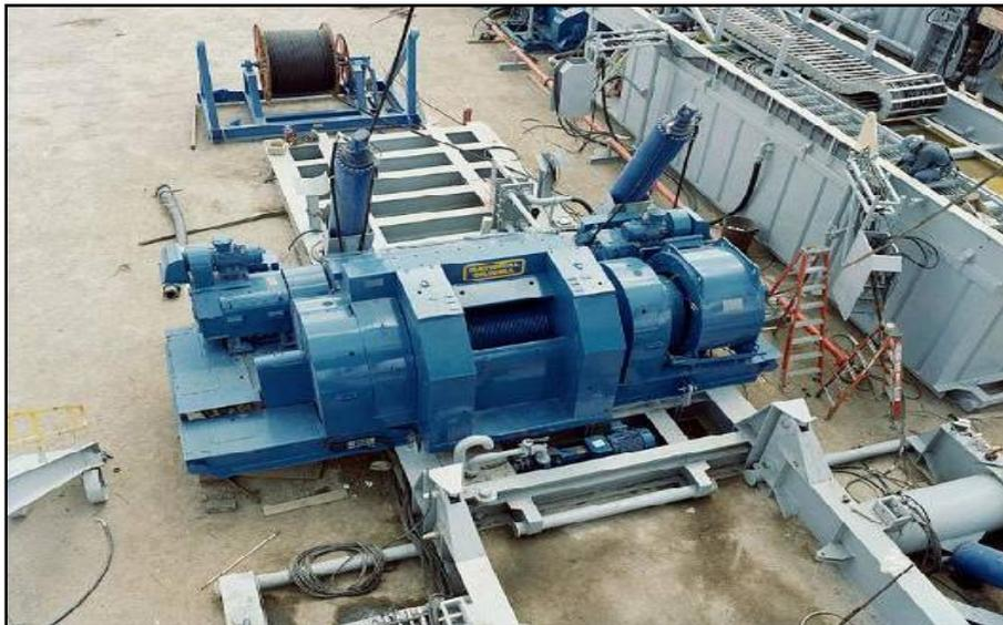
Figure I-11 : Le Treuil De Forage. [1]
