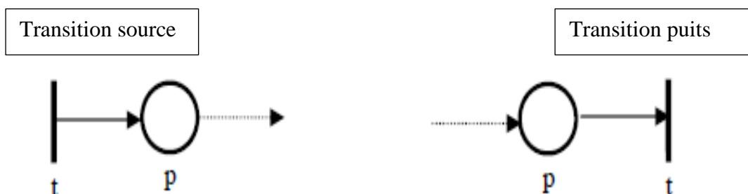
Figure II.3 : Transition source et transition puits.
