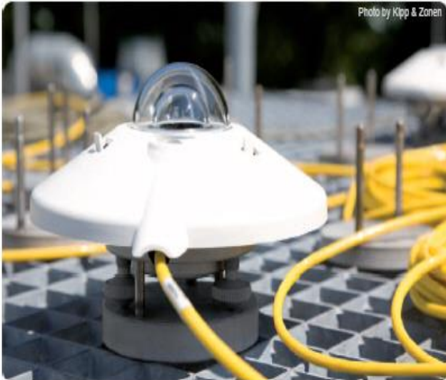
Figure 7. Pyranometer with sun screen
