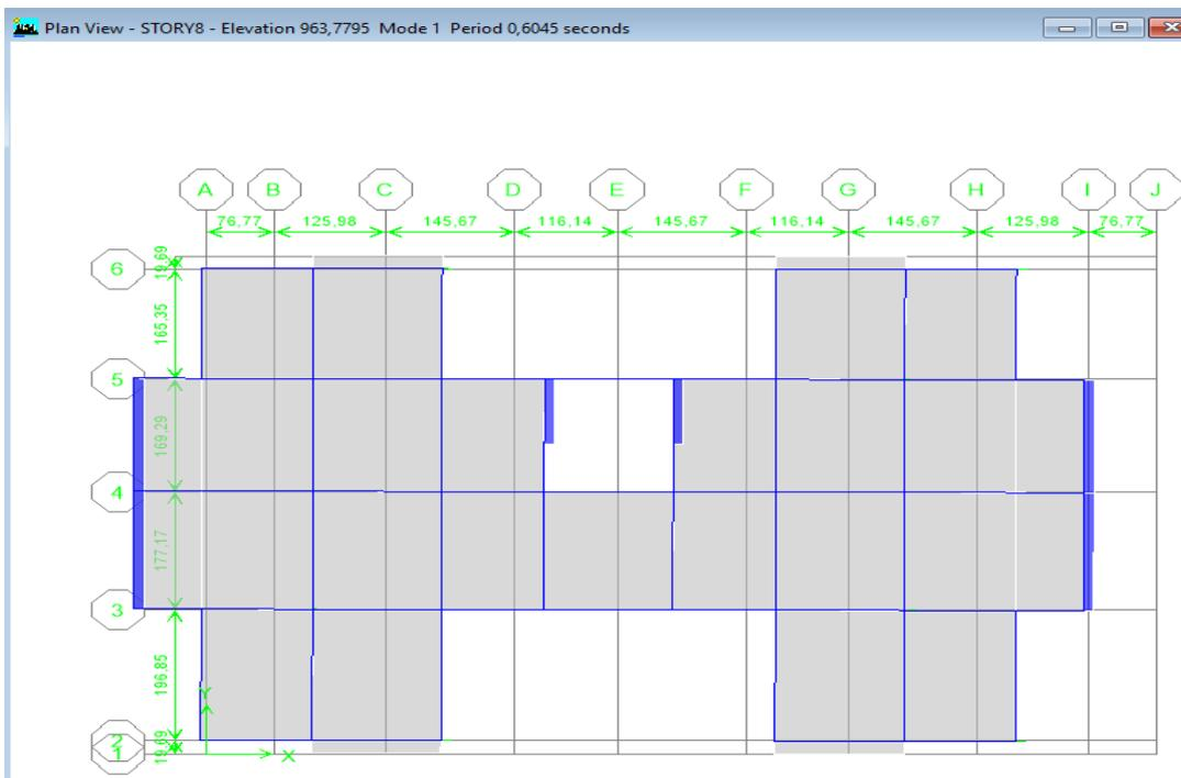
Fig. V.3 Analyse de la structure Mode 1 (translation) T=0,60s
