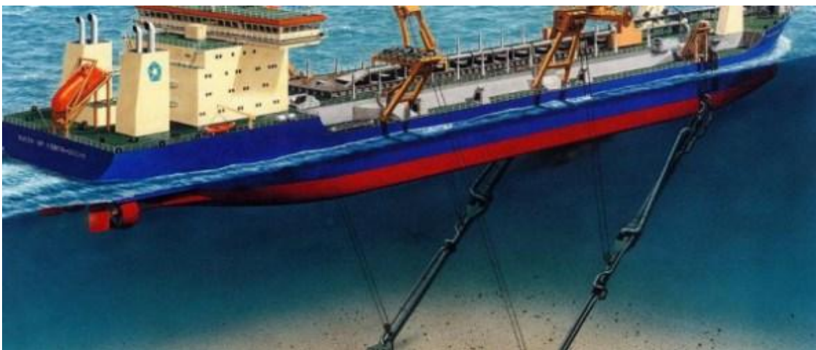
Photo I.4: La drague hydraulique a barrage.
