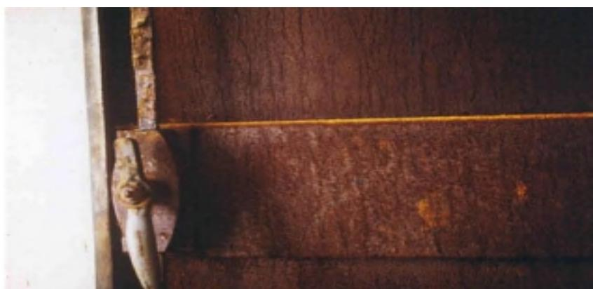
**Figure I.3:** Corrosion uniforme
