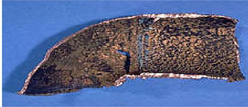
**Figure I-12.** Corrosion érosion /abrasion/cavitation
