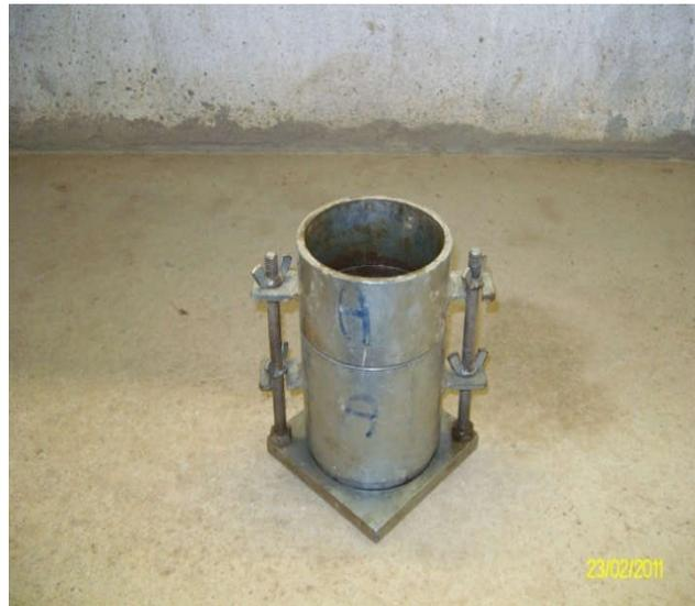
**Figure 0.14: Essai Proctor**
